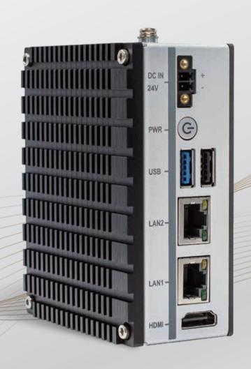
IBX-121 controller supports 16 axes synchronous motion control and integrates ARM 4-core processor that supports multi-core real-time control. It has built in communication protocols such as EtherCAT, Modbus TCP, and OPC UA.IBX-121 controller supports multi-axis synchronous motion control and integrates ARM 4-core processor that supports multi-core real-time control. It has built in communication protocols such as EtherCAT, Modbus TCP, and OPC UA.
