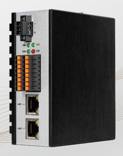
The IBX-111 controller supports simple motion control for up to 8 axes and includes functions for data acquisition, processing, transmission, and device control. The device features one EtherCAT port, one Ethernet port, multiple isolated RS232/RS485/CAN communication interfaces, and supports power failure protection.
